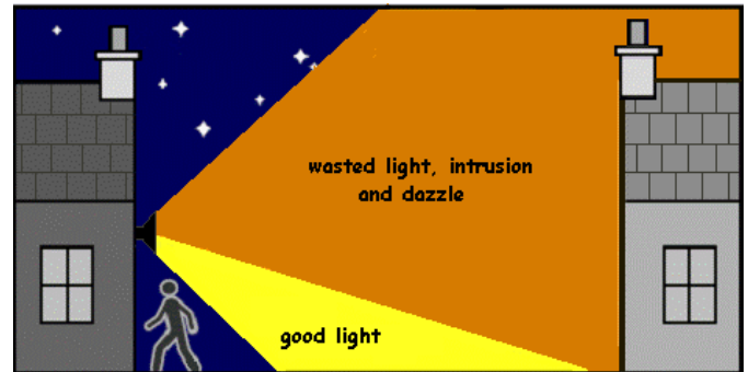
Figure 1: poor positioning and poor direction
